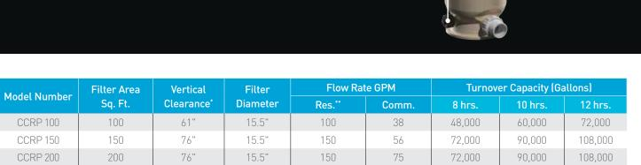
\* Required clearance to remove filter elements \*\* Maximum flow rate
